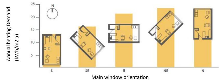
Why Orientation is important, Image from the LETI Climate Emergency Design Guide
